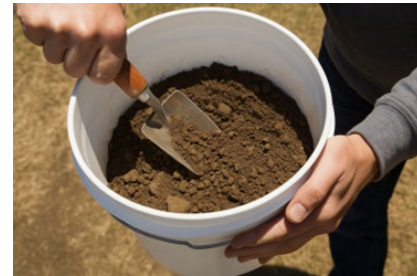
Figure 5. Prepare a composite soil sample by thoroughly mixing the soil and removing plant materials or stones.
