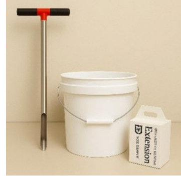
Figure 2. Photograph of a soil probe and proper sampling equipment.
