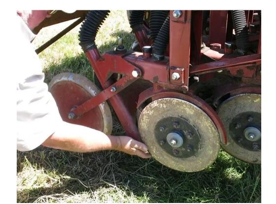
Check all the grease fittings on the unit, and grease if necessary.
