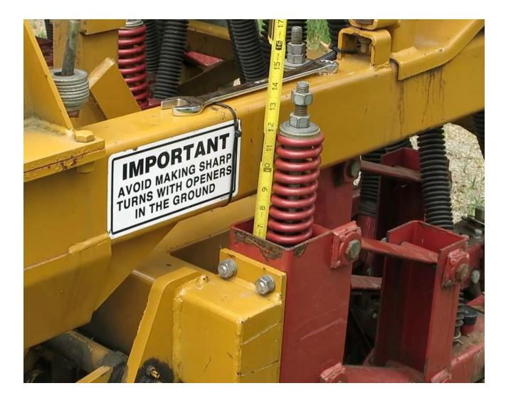
When the drill is properly adjusted, the parallel bars should be level with the ground surface, or slightly higher towards the front of the drill; they should not be higher in the rear. Drive a short distance with the drill lowered and check the depth of the furrow.
