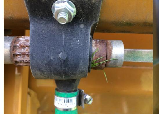
Photos of clogged seed tubes and seed box openings.
