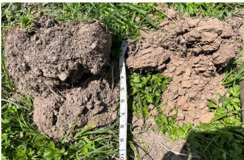
Photo 1. An uncompacted soil (left) compared to a compacted soil (right). These shovel slices were taken from the same field at different locations. You can see the left soil slice is well structured, darker in color, and allows water to move easily into the soil. The right soil slice is poorly structured, lighter in color, and does not allow easy water movement into the soil. Photos are from the author unless otherwise mentioned.
