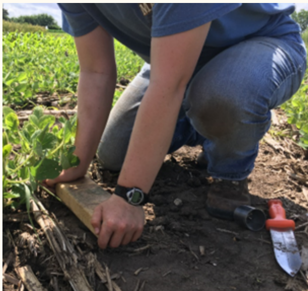
Pressing a bulk density ring into the ground (left) and a collected ring (right)
