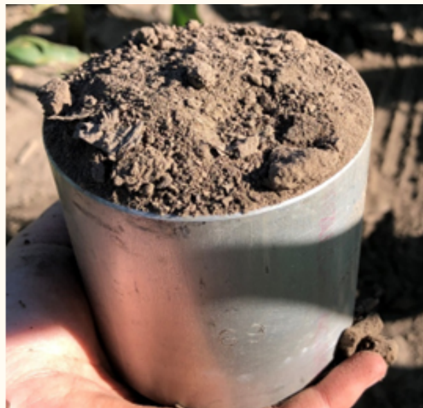
Pressing a bulk density ring into the ground (left) and a collected ring (right)
