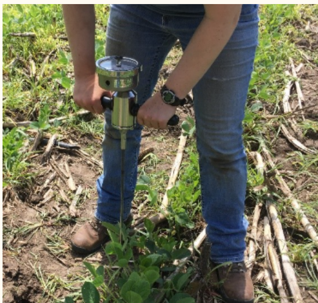
A soil penetrometer being pressed into the soil (left) and a look at the resistance readings (right).
